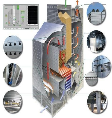
Cut section diagram of the LSU dryer
